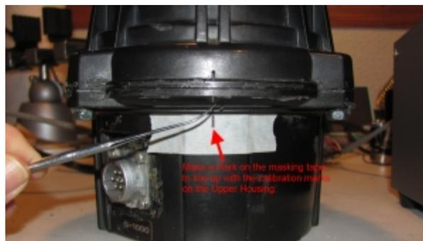
**Step 2:** Put a piece of masking tape on the Lower Housing (item #1 in the Service Manual) and mark the position of the rotor with the alignment marks on the Upper Housing (item #2 in the Service Manual).
