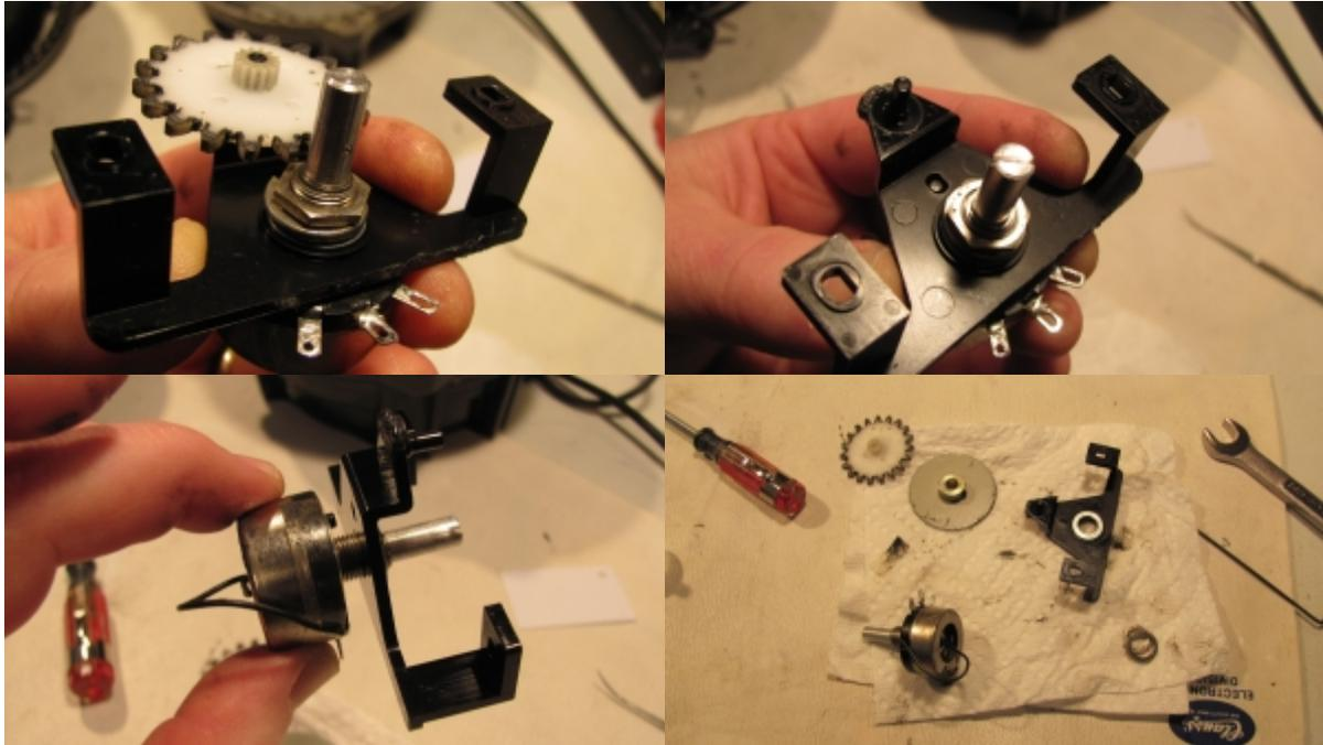
**Step 10:** Next you must remove the pot from the assembly and mount the new one in its place.
