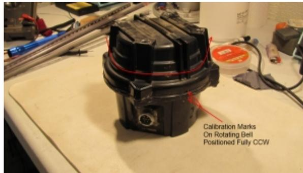
**Step 1:** Operate the rotor to its fully CCW position.
